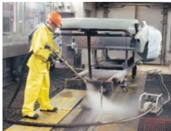
Carrier Cleaning - With an NLB rotating lance, an operator can strip away hardened paint and dirt from skids and carriers.
