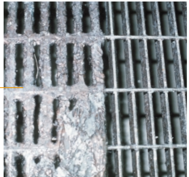
Typical paint booth grate before and after SPIN JET® cleaning.
