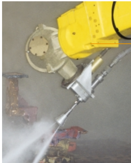
Ultra-high pressure rotating nozzle, directed by a robot, follows a programmed path.
