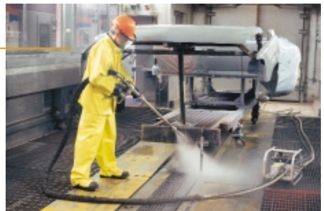
An operator with a hand lance (ultra-high pressure shown) makes short work of build-up on an automotive carrier.
