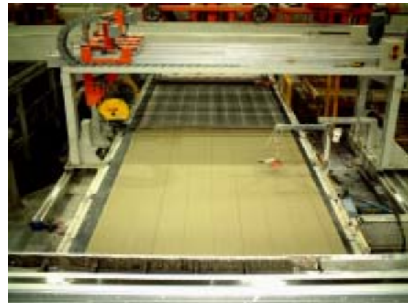
A single large sheet has been cut into eight individual pieces of siding.
