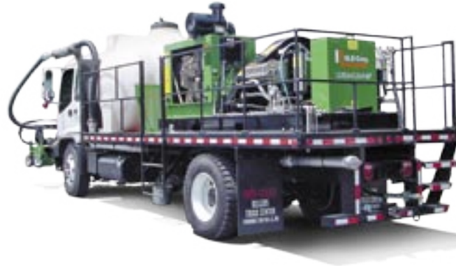
STARJET™ system with: extra-large water tank, and 24" nozzle assembly, and on-board vacuum recovery with debris separation
