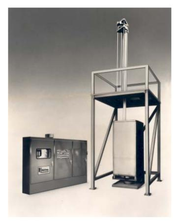
platform. The end of the lance features an articulating nozzle mechanism with a swing of 120-degrees to insure complete cleaning coverage inside the tote. Also, the lance moves along an x-y axis while inside the tote to enable the nozzle to reach far into the top and bottom corners. The automated tote cleaning system reduced cleaning time to 30 to 60 minutes per tote.
