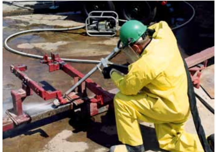
Paint removal for automotive skids using the NLB Model NCG8450A-3 rotating hand lance.
