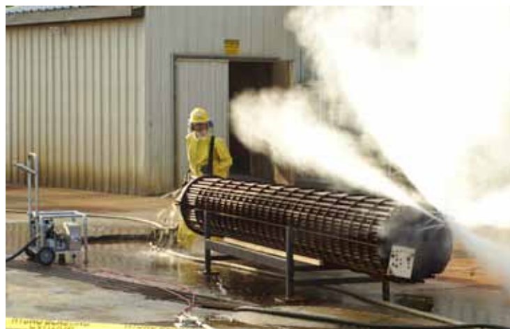
The Saflex-2000's high torque flex lance drive system makes cleaning tube bundles fast and easy.
