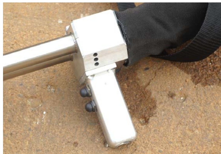
The ergonomic hand lance features simple controls. One button feeds the lance in, and the other pulls the lance back out.
