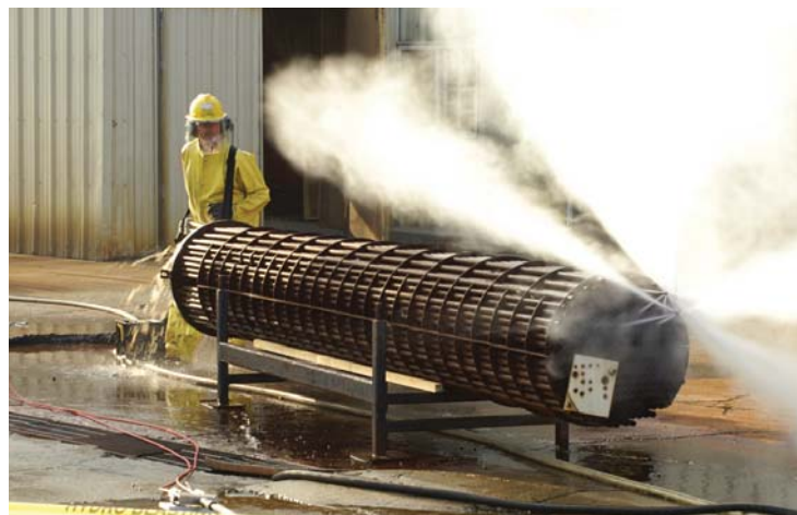
The Saflex 2001's high torque flex lance drive system makes cleaning tube bundles fast and easy.
