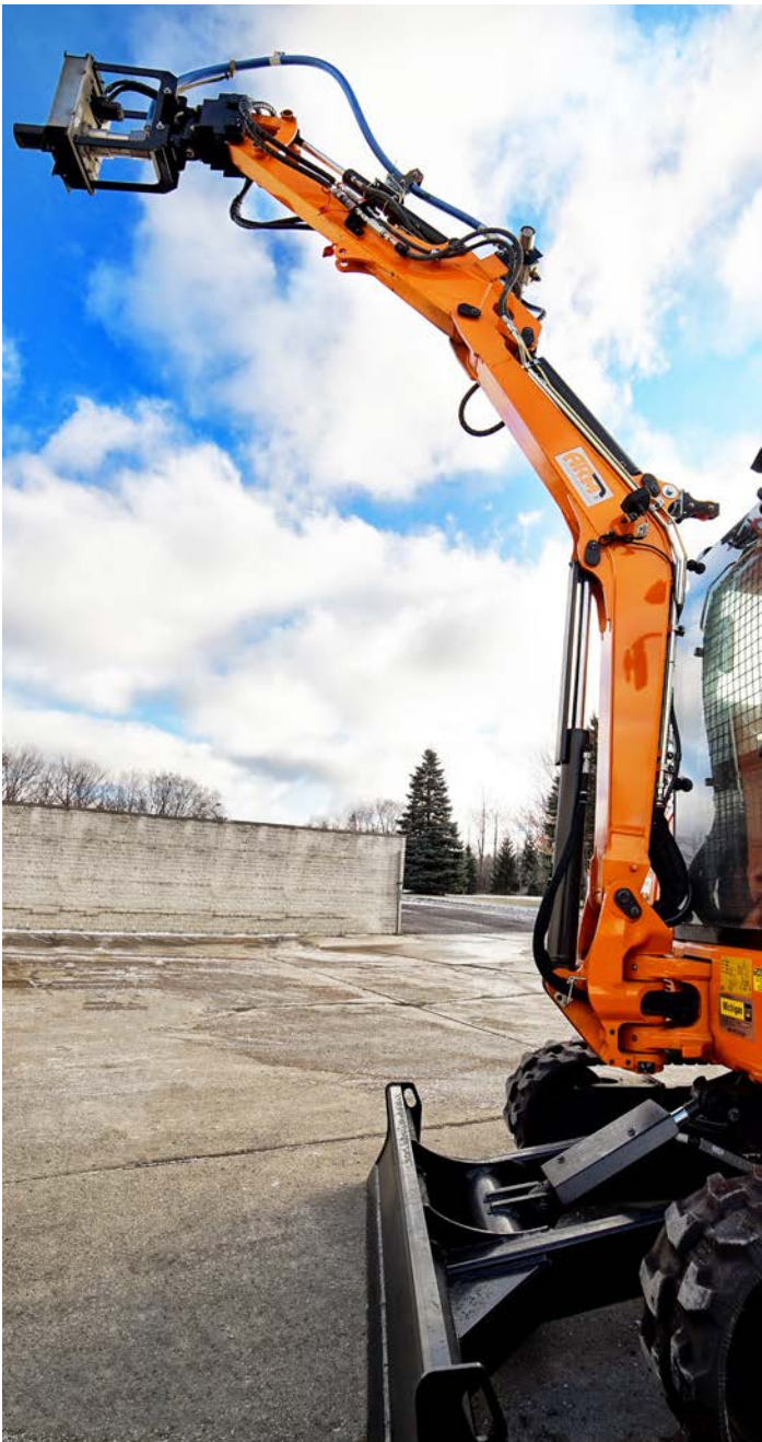
The NLB ARM allows operators to bring 40k psi to difficult to reach places.
