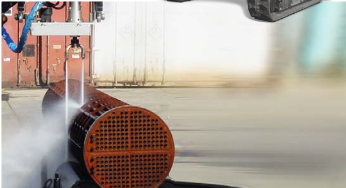
An available rotating jetting head is ideal for cleaning tube bundles and surfaces with draws and multi-level surfaces.
