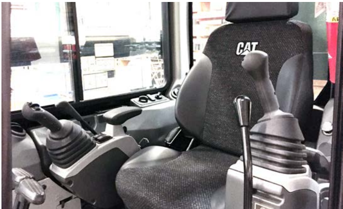
A safe and dry climate controlled cab for the operator with integrated speed and rotation controls.
