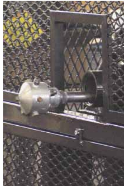
NLB P-10 Line Mole Nozzle attached to the Roto-Reel for optimal pipe cleaning.
