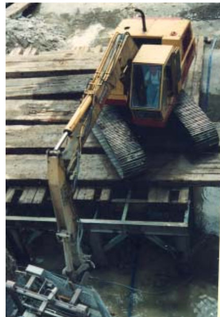
The NLB X-Y unit attaches easily to the arm of an excavator.
